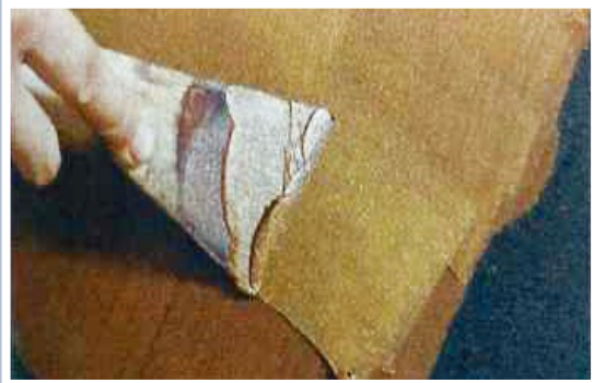
Lacquer is applied to the base frame and adhered burlap (hemp cloth) to it then painted with Shell powder
